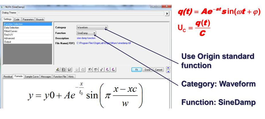
Fitting function ; y0,A,t<sub>0</sub> xc, w – fitting parameters
