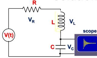
Vc ~q, fiiting function:  $V_c = V_{co}(1+at)e^{-at}$
